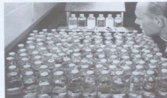
FIGURE 15.12 Testing compatibility of rubber closures with a solution. (Courtesy of Abbott Laboratories.)
